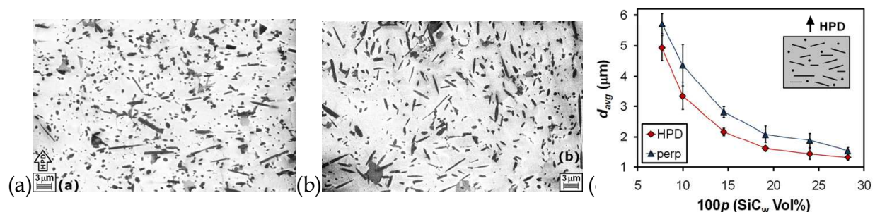
Fig 7. Scanning electron micrographs of the microstructure for an \text{Al}_2\text{O}_3\text{-SiC}_w sample containing 14.5 vol% \text{SiC}_w . In (a), the white arrow points along the hot-pressing direction. In (b), the microstructure is viewed along this direction. Part (c) shows the average distance between \text{SiC} inclusions along the HPD and perpendicular direction. The inset shows a schematic of the microstructure. Source: Bertram & Gerhardt, 2010.
