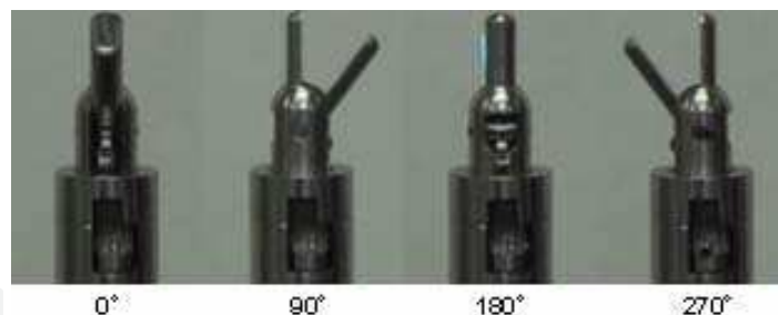
Fig. 9. Transition chart of the rotary gripper
