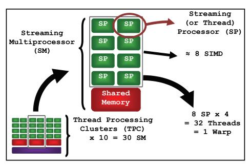
Fig. 2. Simplified architecture of an Nvidia Tesla 10.
