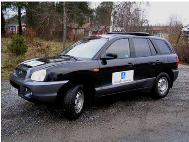
Fig. 2. Photo of the measurement car including the antenna solution with an extra disc as ground plane, used by the Swedish regulator, PTS
