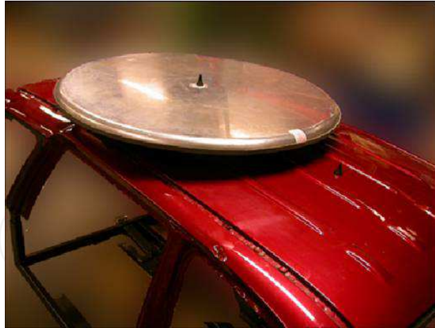
Fig. 4. Photograph of the measurement antenna solution with an extra disc added on top of the car
