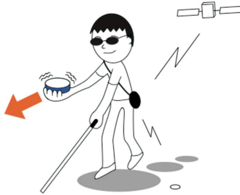
Fig. 5. Overview of kinesthetic navigation for pedestrians with visual impairments. After location data received from a satellite system or embedded sensors and orientation data had been collected and processed, a haptic cue of direction was presented to the pedestrian
