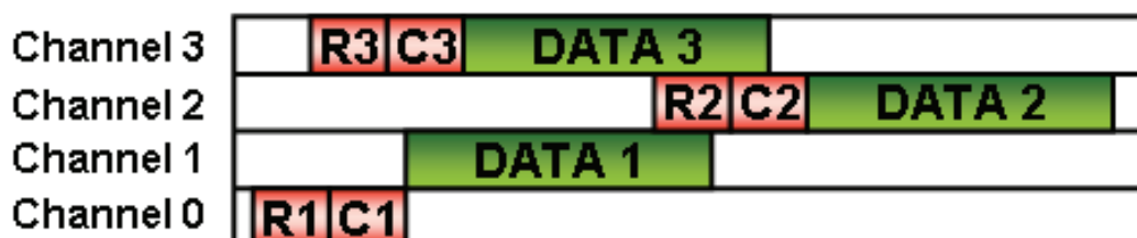
Fig. 5. Common Hopping Approach (figure inspired from [mo07])
