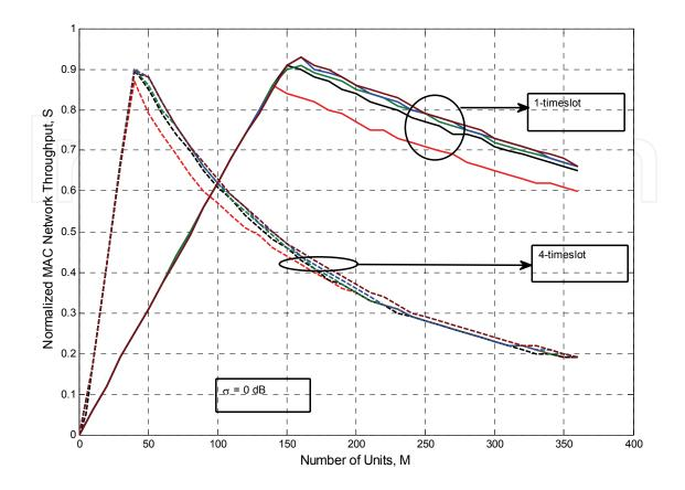
Fig. 14. Normalized Average SOC-MAC Network Throughput for  $\sigma$  = 0 dB, and MAX\_TIMEOUT = [2, 4, 6, 8, 10]
