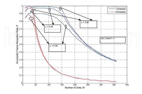
Fig. 11. Successful Packet Reception Rate versus Number of Units for MAX\_TIMEOUT = 4, and  $\sigma$  = 2 dB, 4 dB and 8 dB
