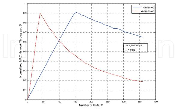
Fig. 10. Normalized Average SOC-MAC Network Throughput versus Number of Units for MAX\_TIMEOUT = 4, and  $\sigma$  = 0 dB
