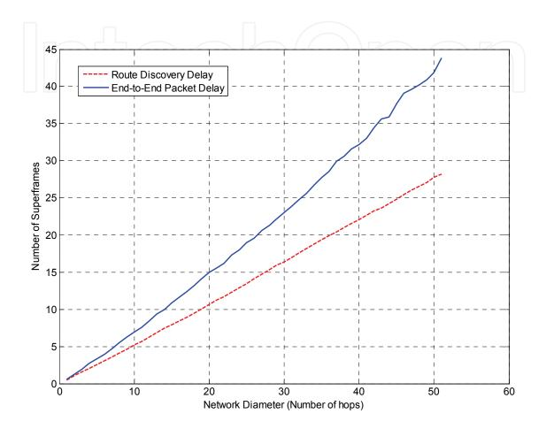
Fig. 15. Route discovery and End-to-End Packet Delay
