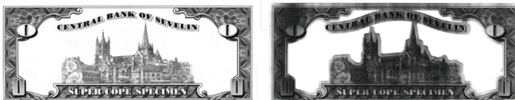
Fig. 9. Wiping error (right) in an intaglio printing process (Glock et al., 2011).
