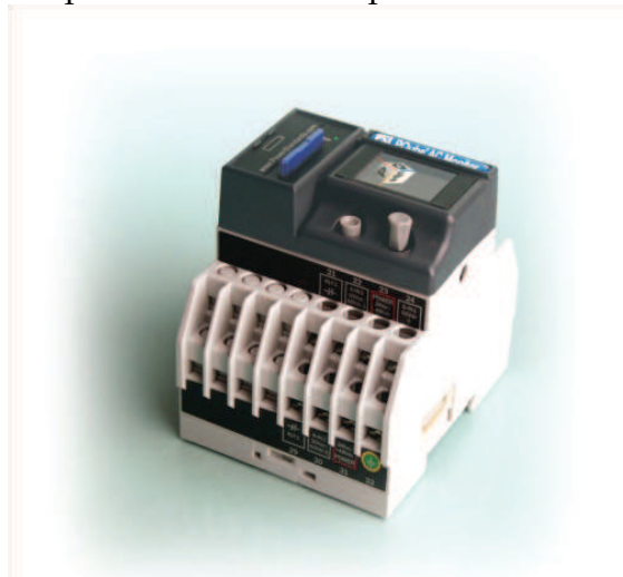
Fig. 4. Prototype of the three-phase, voltage-and-current, 61000-4-30 Class A power quality monitor. The digital camera influence can be seen in the SD memory card, which holds up to 2 000 MB of data. Standard DIN-rail mounting means installation is cheap and quick.
