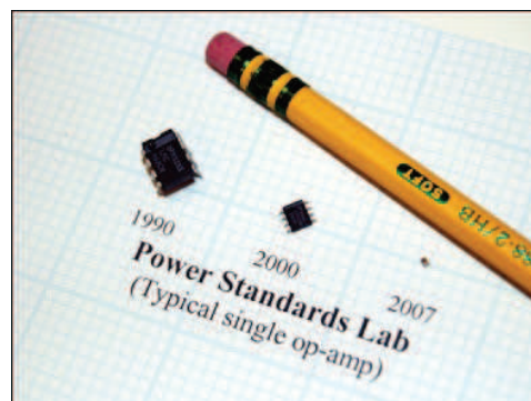
Fig. 1. Reduction in component size. Smaller components reduce costs in several ways: smaller printed wiring boards, smaller plastic packages, even smaller power supply requirements. The packages shown are, from left, through-hole DIP, surface mount, and BGA or ball-grid-array.
