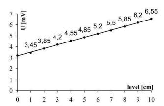
Fig. 19. SPCE response versus the petrol level
