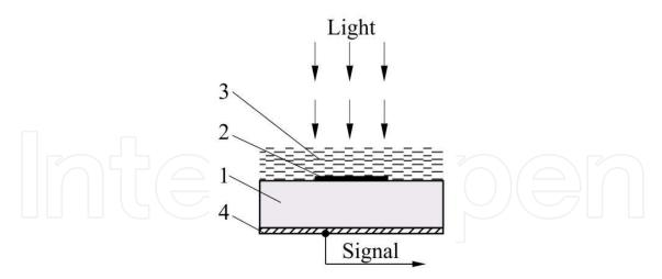
Fig. 17. Setup for the observation of SPCE at liquid-sold interface: 1-solid, 2-solid-liquid interface, generating the signal, 3-fluid under study, 4-electrode
