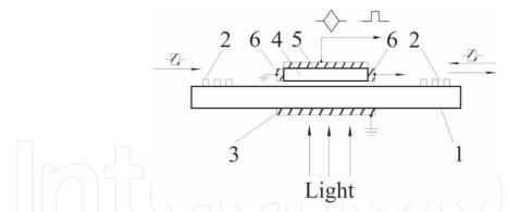
Fig. 1. Testing structure for acoustoelectric interaction: 1 – piezoelectric; 2 – SAW transducer; 3 – bottom electrode; 4 – semiconductor; 5 – top electrode; 6 – electrodes for detection of the longitudinal acoustoelectric effect
