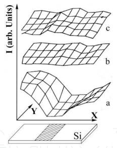
Fig. 12. Response distribution for a silicon plate. The scanned area along the x-axis is ca. 4 mm and the width of the scratched (hatched) area is ca. 2.5 mm; laser beam intensity:  $a-30\mu W$ ,  $c-700\mu W$
