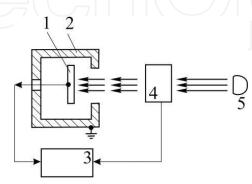
Fig. 5. Experimental setup: 1-specimen, 2-screen, 3-measuring device, 4-modulator, 5-light source
