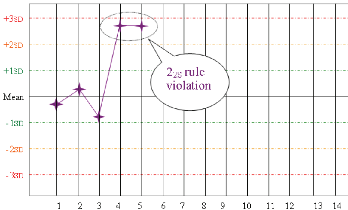
Fig. 4. Rule 2_{2s} - reject the run when 2 consecutive controls exceed the mean \pm 2s .
