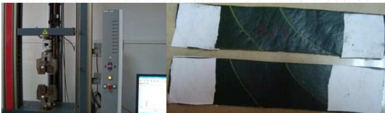
Fig. 10. The tension test of plant leaf
