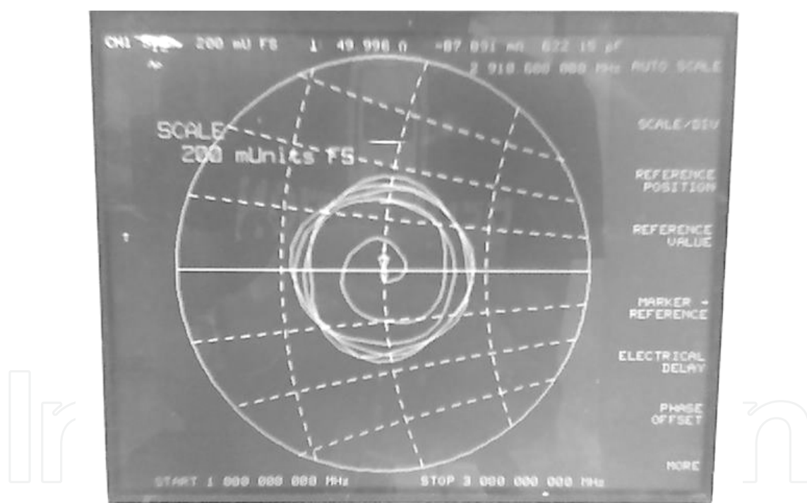
Fig. 8. Measured Input Impedance of DRA Structure.
