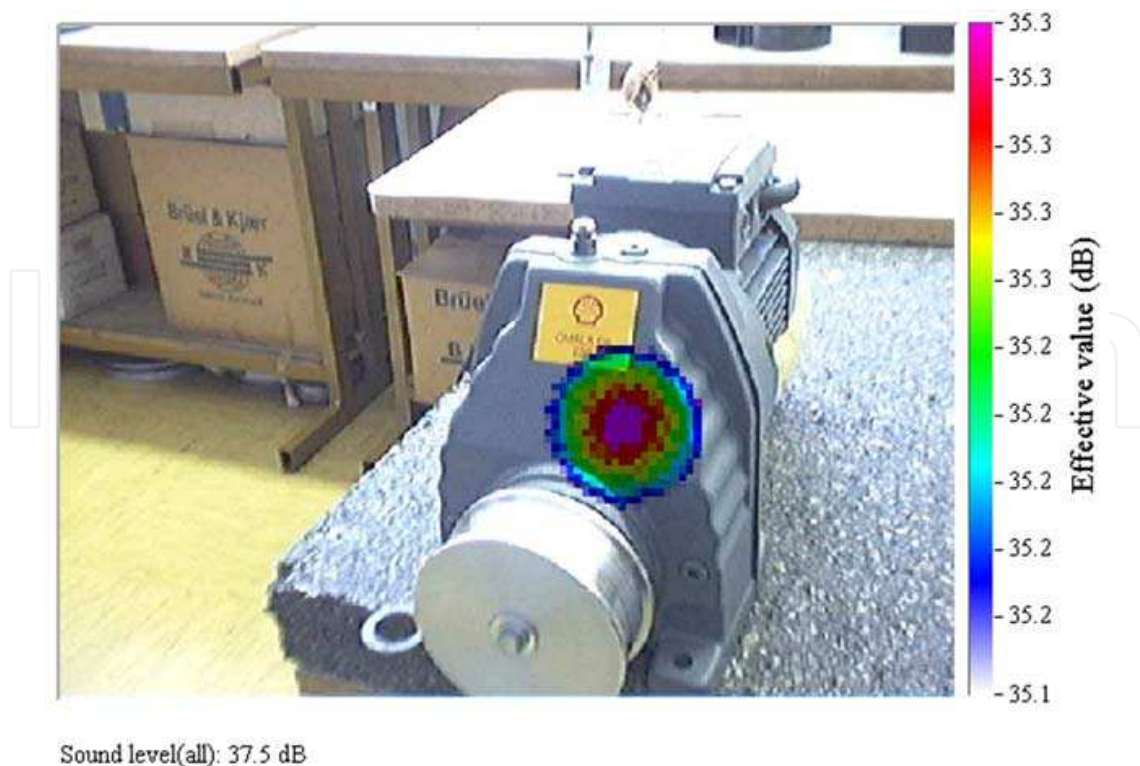
Fig. 5. An acoustic image with noise source of a gear unit of a faultless gear
