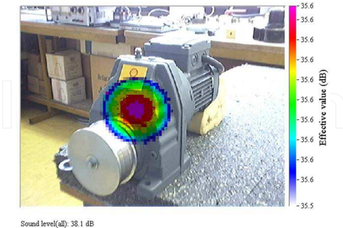
Fig. 7. An acoustic image with noise source of a gear unit with a crack in the tooth root
