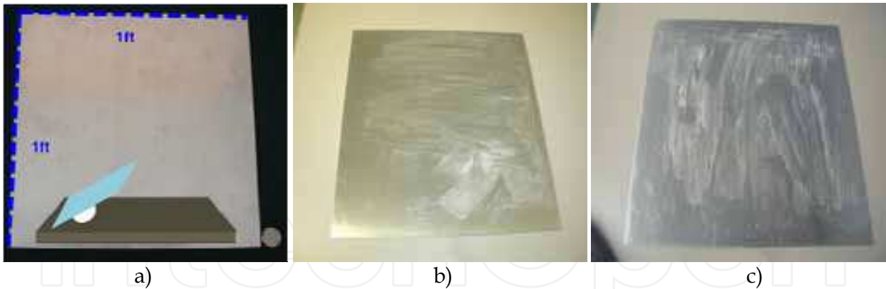
Fig. 2. Sample preparation: (a) Clean Al plate ready for sample smearing technique; (b) 50 µg/cm² of TNT loading concentration; (c) 100 µg/cm² of TNT surface concentration
