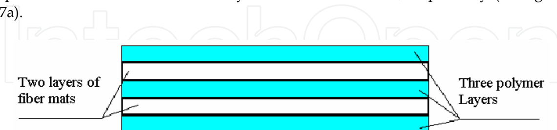
Fig. 12. Sandwich structure of PLA and fibril composites for compressive molding
