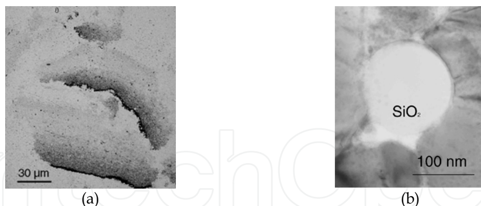
Fig. 16. Hot compacted plasma arc powder (a) and silica particle at grain boundaries (b)
