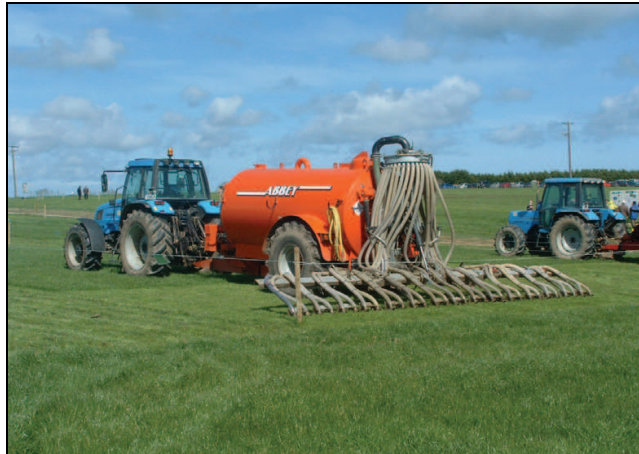
Photo 3. Slurry tanker with trailing shoe application system (Source: Teagasc)
