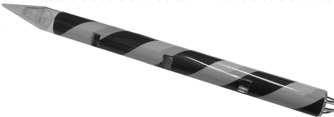
Fig. 9. Magnetic resonance probe used to determine the ratios of particulate and biological clogging. This version has three sensors spaced along its length.
