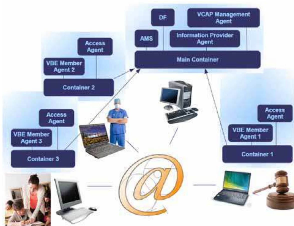
Fig. 9. Distributed structure of the VCAP platform
