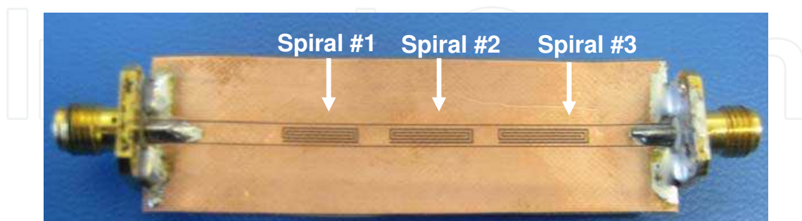
Fig. 15. Photograph of manufactured CPW 3-bit multiresonator on 90 \mu\text{m} Taconic TF-290 substrate.
