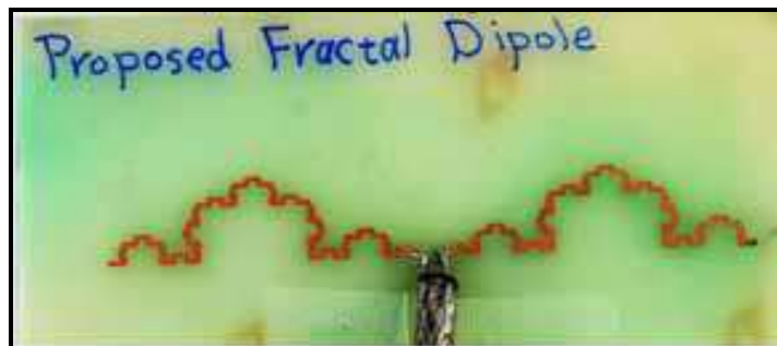
Fig. 10. Photograph of the fabricated (P3) antenna
