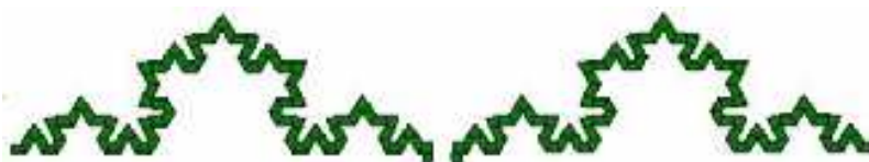
Fig. 5. Standard Koch fractal dipole antenna.
