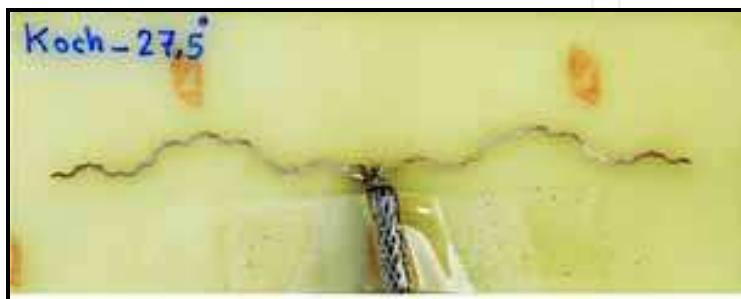
Fig. 9. Photograph of the fabricated K3-27.5° antenna.
