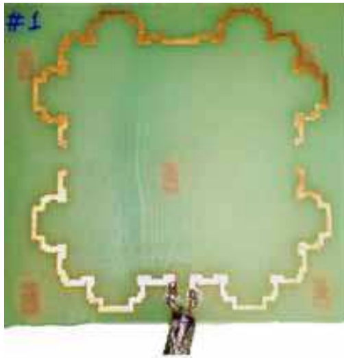
Fig. 27. The Fabricated Fractal Loop Antenna.
