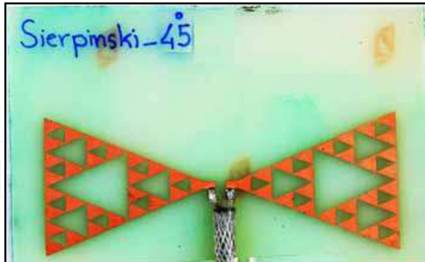
Fig. 18. The fabricated S3-45° antenna.
