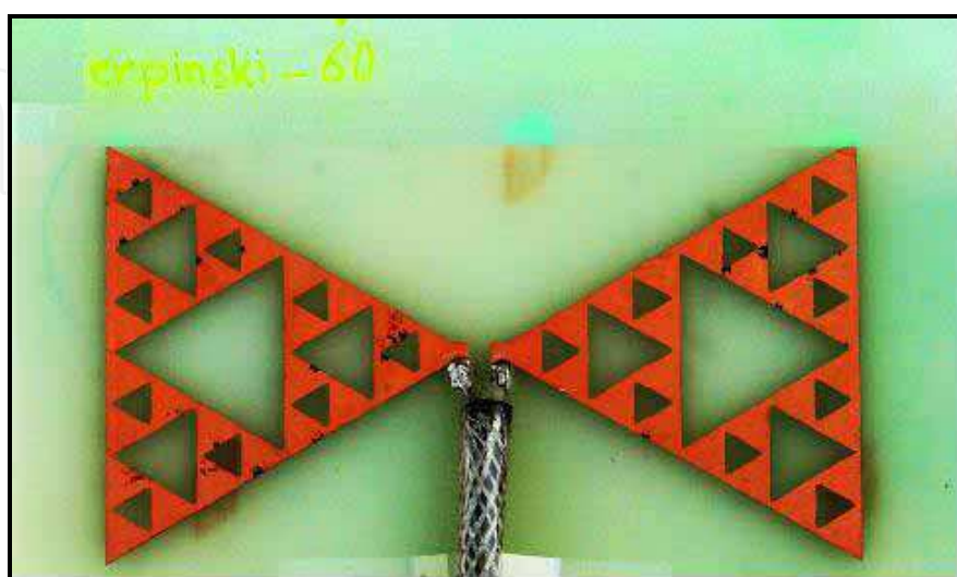
Fig. 17. The fabricated S3-60° antenna.
