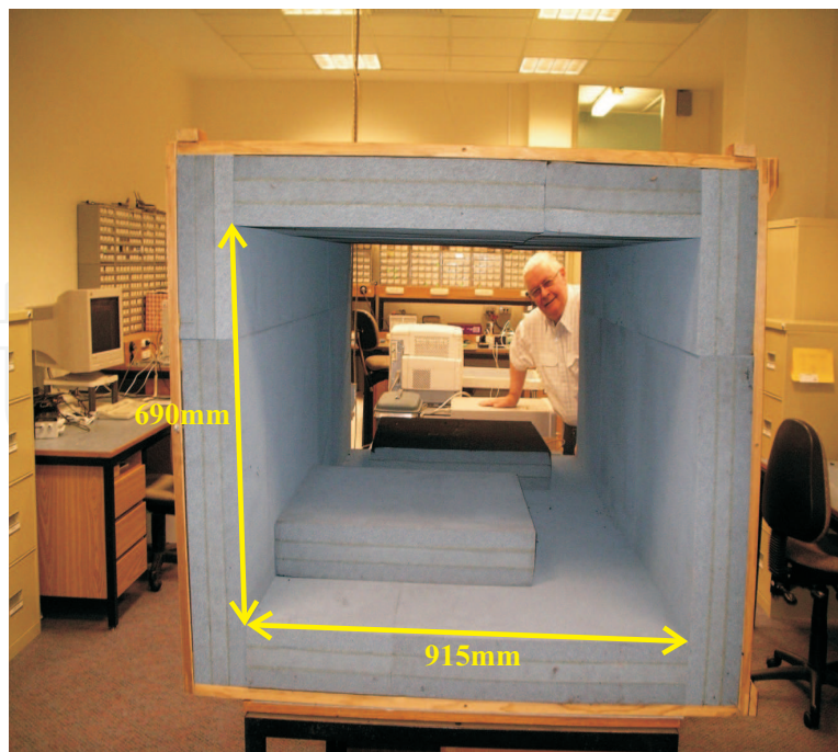
Fig. 8. A shielding tunnel.
