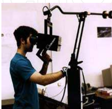
Fig. 2. A Binocular Omni-Orientation Monitor (BOOM)
