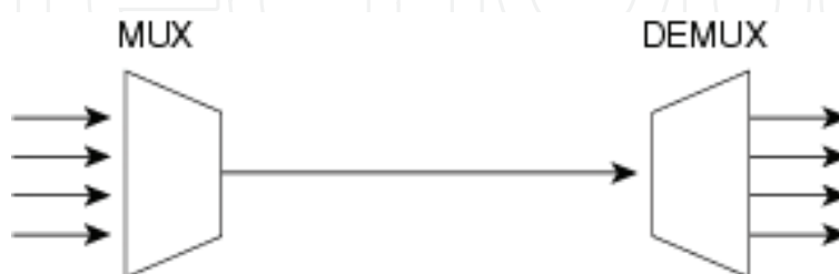
Fig. 1. Multiplexing and Demultiplexing operations.
