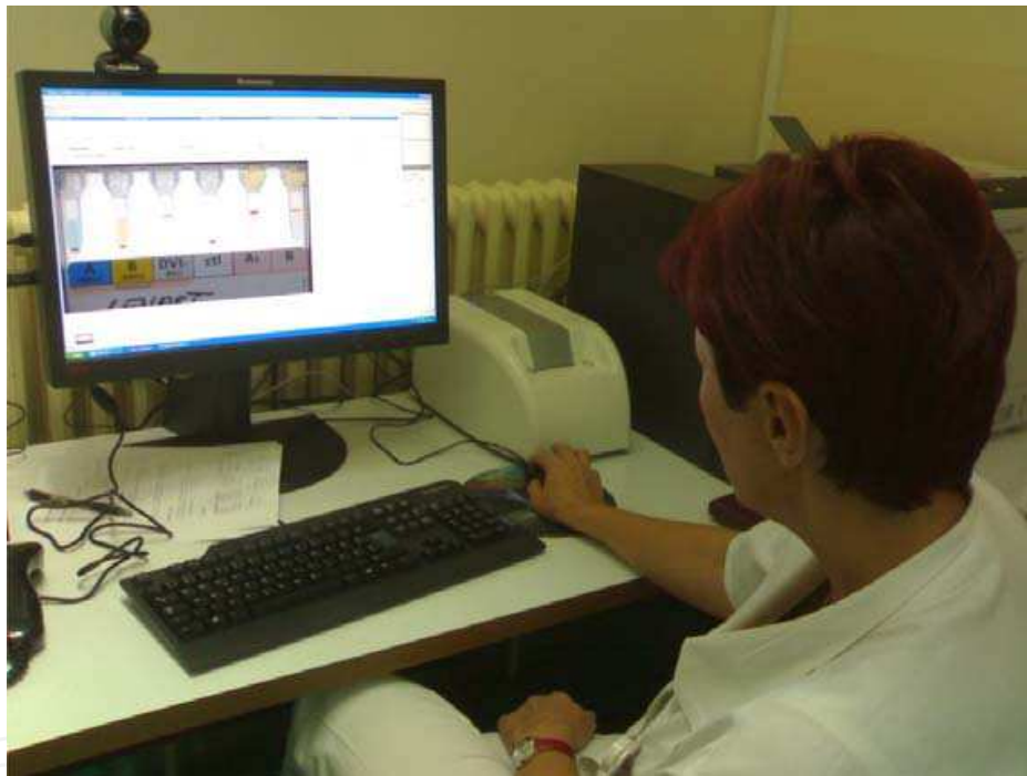
Fig. 3. Laboratory setup of the telemedical system. Main application window can be observed on the terminal. Gelscope device is visible right next to the terminal monitor. Videoconference call is not established.
