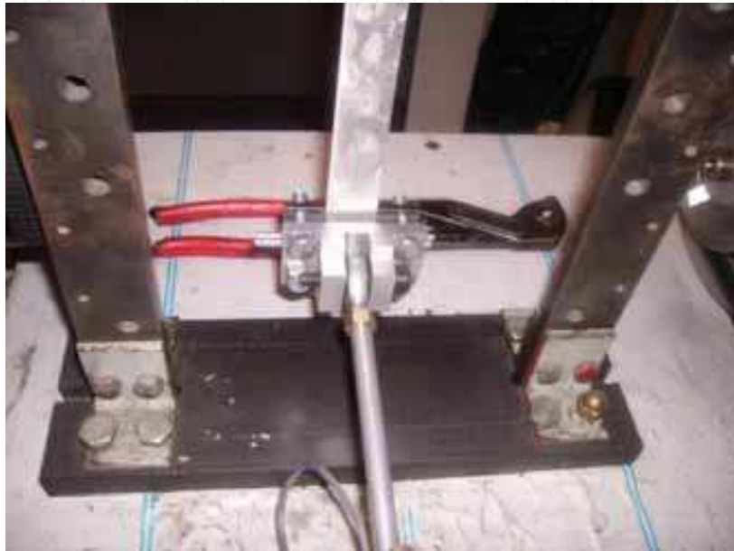
Fig. 22. System grasping between specimen and machine
