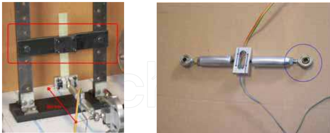
Fig. 4. Control system through horizontal beam (on the left) and joint (on the right)
