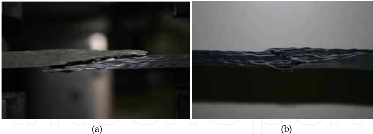
Fig. 6. Joint failure (a) through interface (b) across the joint cross-section
