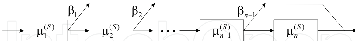
Fig. 1. Diagram of phases of a n -th order Coxian distributed service time
