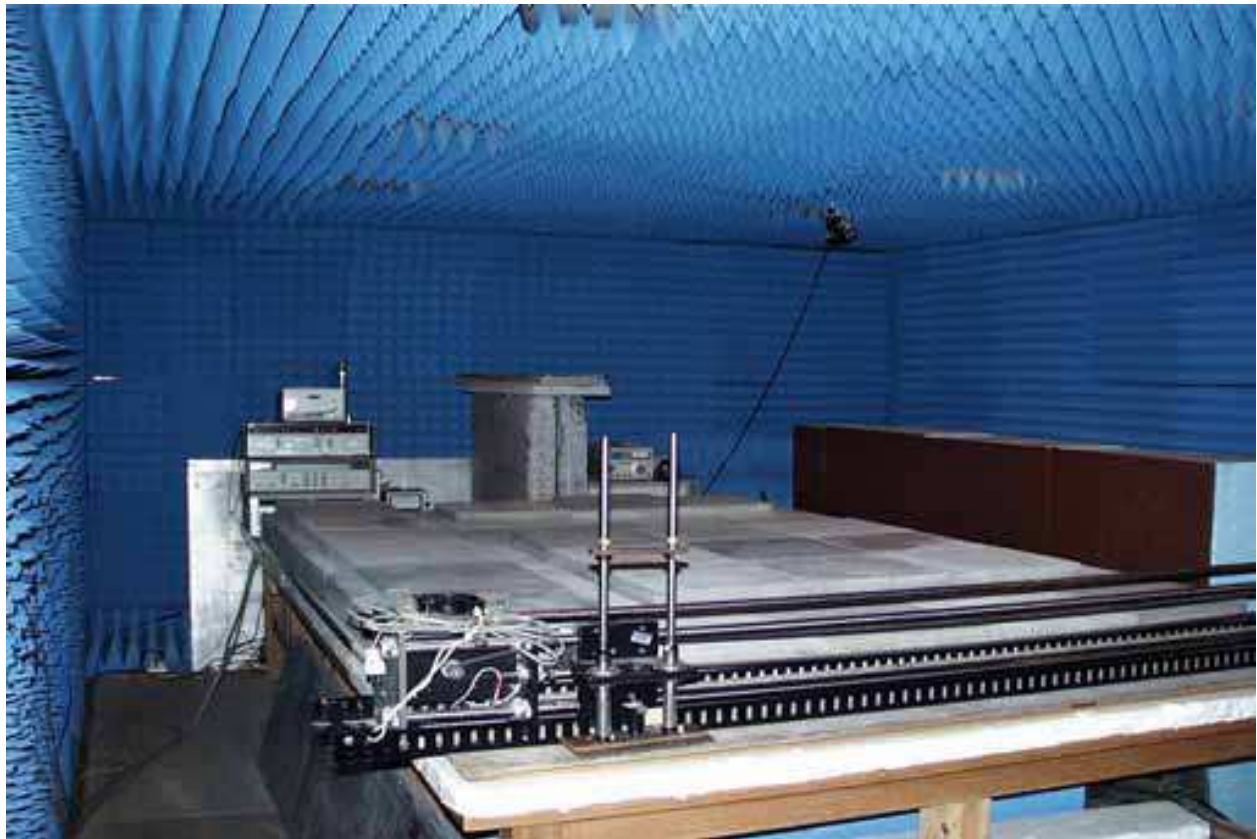
Fig. 3. A photograph of measurement system inside our radio-frequency anechoic chamber
