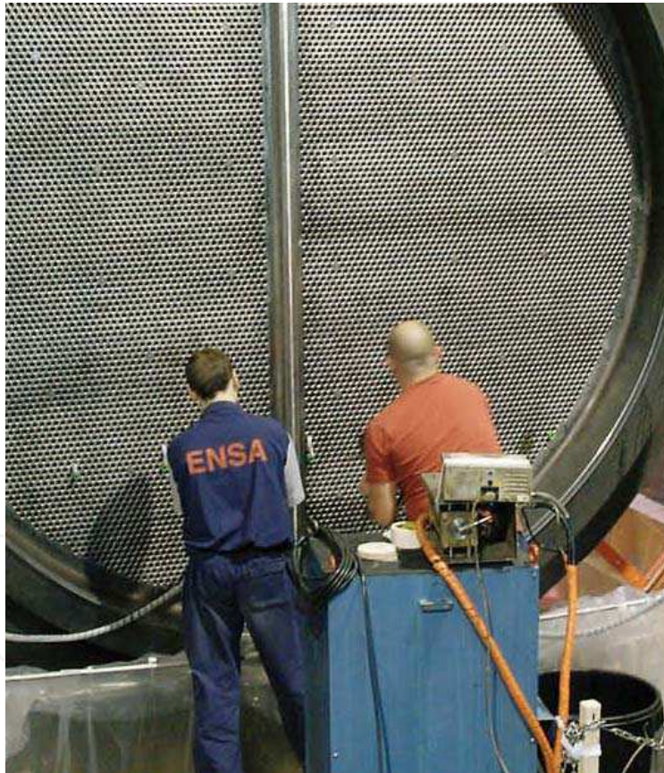
Fig. 1. Tubesheet of a steam generator for the nuclear industry
