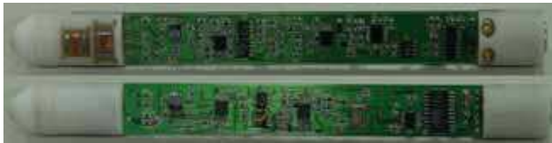
Fig. 11. Photograph of the new probe, front side (above) and rear side (bottom)
