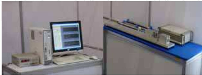
Fig. 12. Photograph of the completed measuring system data acquisition software in PC and probe scanning system
