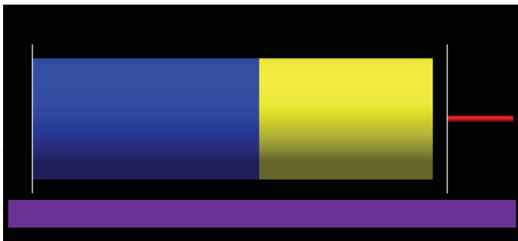
Fig. 16. Moderator’s assembly: copper layers (white), Fluenta TM material (blue), iron (yellow), plasma column, producing neutrons inside the DPF discharge chamber (red)
