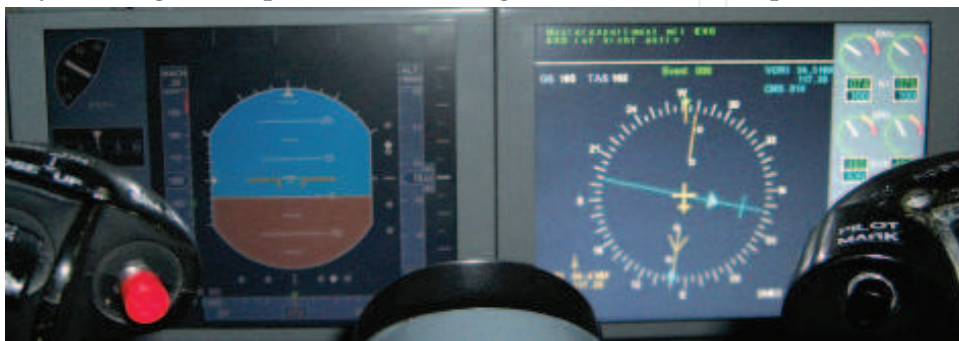
Fig. 2. Typical primary flight display and navigation display
