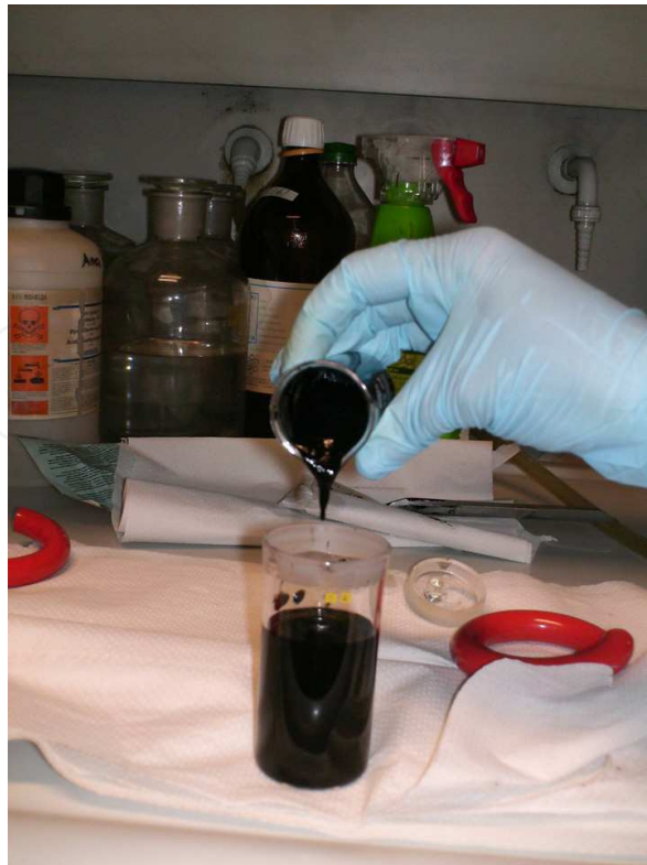
Fig. 1. Filling a thermal conductivity cell with the ionanofluid [\text{C}_4\text{mim}][(\text{CF}_3\text{SO}_2)_2\text{N}] + 0.5\%(\text{w/w}) MWCNTs.
