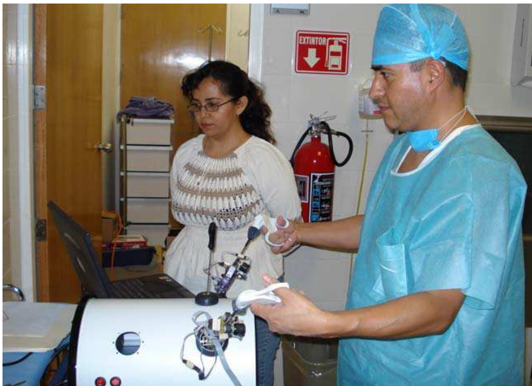
Fig. 4. General set up of the instrumented trocar installed in the trainer. The image shows the arrangement during the training.
