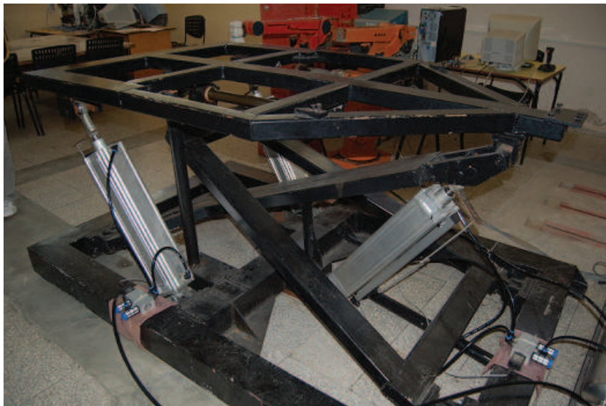
Fig. 1. SIMPRO 3DOF pneumatic driver simulator parallel platform
