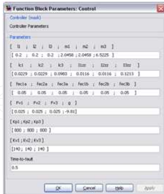
Fig. 12. Window for entering controller parameters
