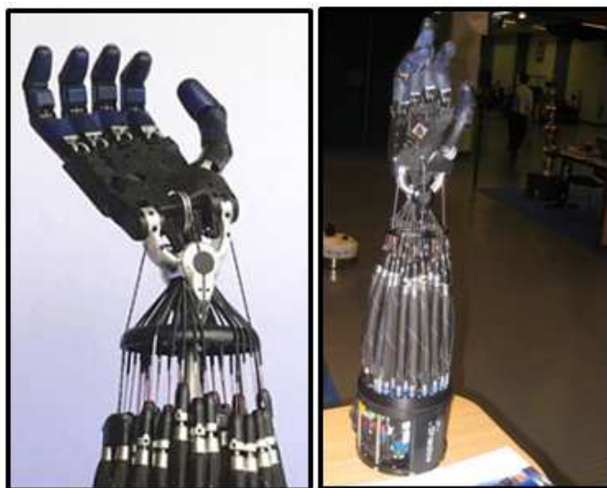
Fig. 6. The Shadow hand actuated with air muscles
