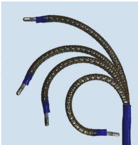
Fig. 4. A continuum manipulator with tendon actuation
