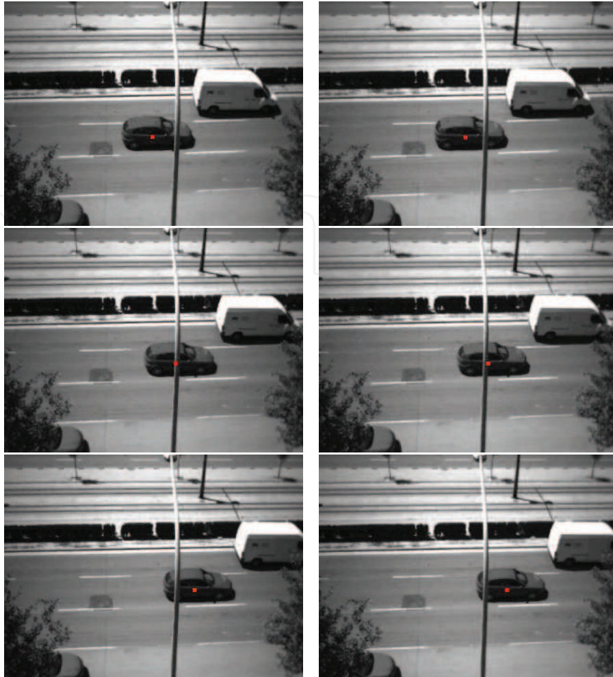
Fig. 21. RLS tracking stereo in a real sequence
