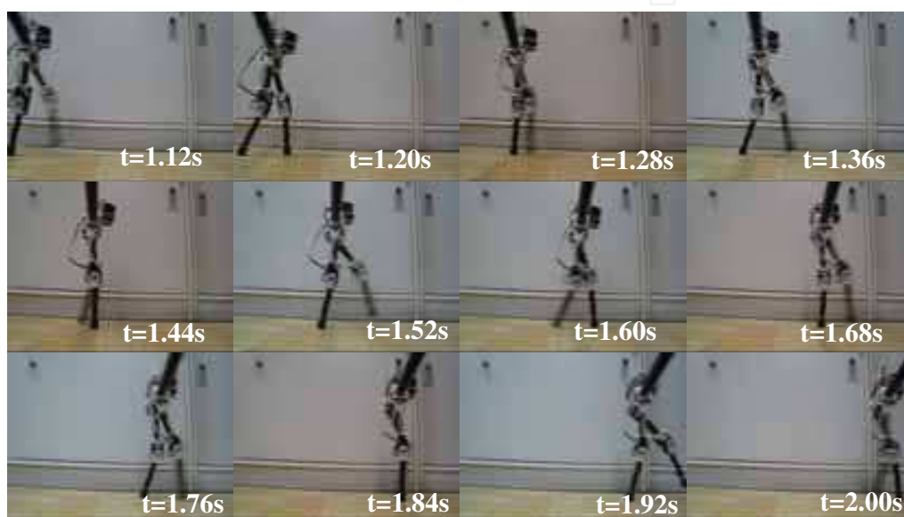
Fig. 17. Video frames of THR-I taking four consecutive steps with \delta = 0.89 . The robot is walking at 0.20 s per step
