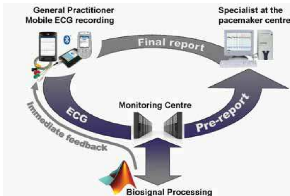
Fig. 5. Magnet effect based device checks consisting of mobile ECG recording units at the general practitioner, a monitoring centre with biosignal processing units and reviewing units for specialists at the pacemaker centre.
