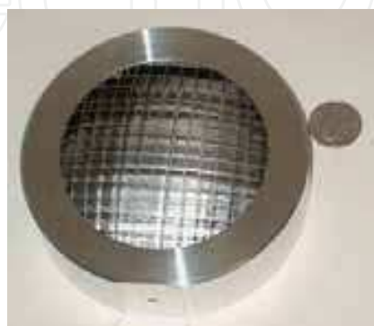
Fig. 7. Illustration of lobster eye, developed at Physical Optics Corporation. The biological lobster eye also has reflection channels with square-cross-sections
