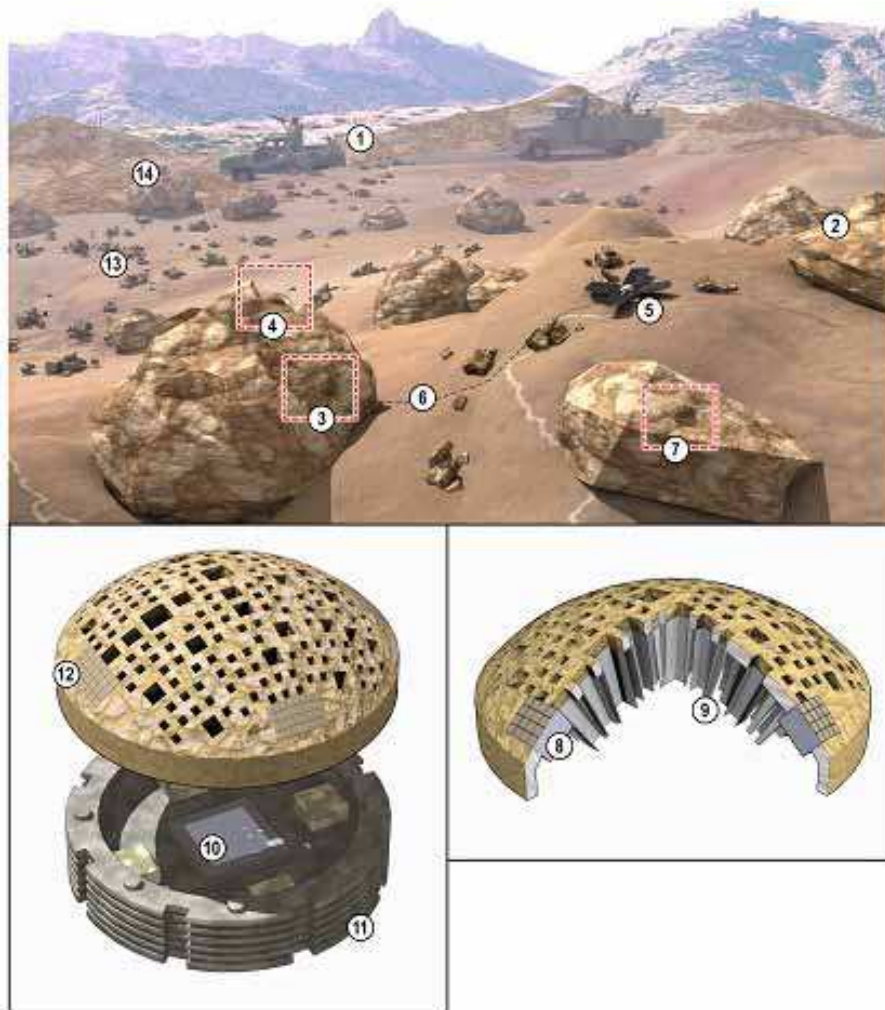
Fig. 11. Camouflaged hemispheric lobster-eye awareness sensor, including: (1) IR target; (2), (3), (4), (7) lobster eyes; (5) remote solar panel that can be charged all day to provide electrical energy for all-night operation (in the stationary case); (6) power cable; (8), (12) local solar batteries; (9) metallic waveguide; (10) focal plane array (FPA); (11) sensor housing; (13), (14) sensor “rocks” dropped from the air
