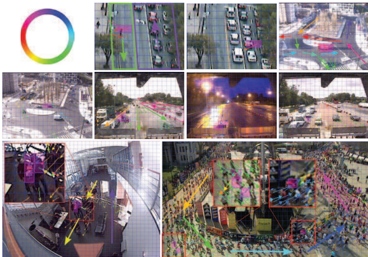
Fig. 16. Example of detection such as jaywalkers, wrong way movement, car pulling out or chaotic movement due to people argument, etc. All the arrows respect the color legend given in the first on the top left image. Ground truth for each scene is represented with large arrows.
