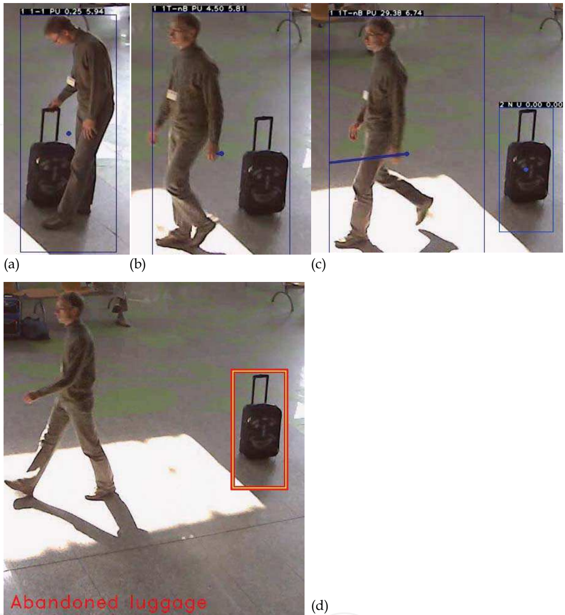
Fig. 14. An example of abandoned luggage detection: (a) initial state, (b) detected left luggage, (c) detected person away form luggage, (d) detected luggage still unattended, high-level event 'abandoned luggage' detected, visual alert
