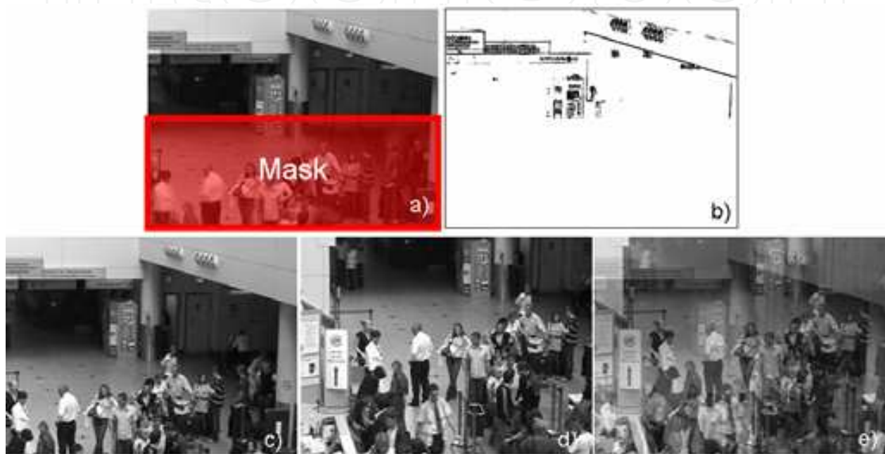
Fig. 18. Example of diagnostic function. The figure a) shows a “standard” scene, that contains its invariant elements (in this case the upper part of the image). The figure b) shows the gradient of the background after applying the binary threshold. Figures c) and d) show the scene before and after the shift of the camera and in figure e) the result of the comparison.
