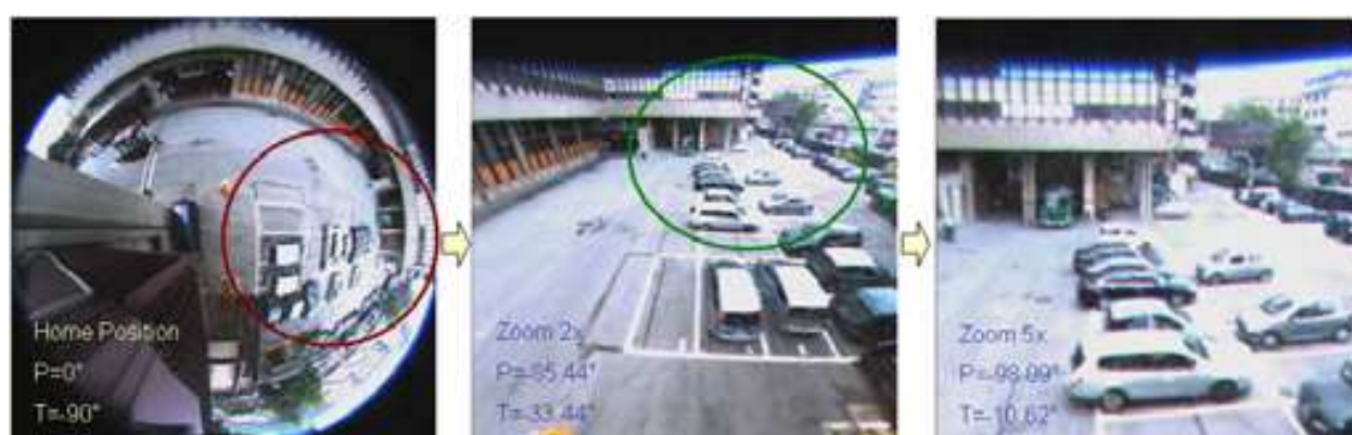
Fig. 14. Example of a virtual PTZ. On the left a fisheye image. In the middle and on the right the prospective projections of the circled areas, based on the pan, tilt and zoom parameters.
