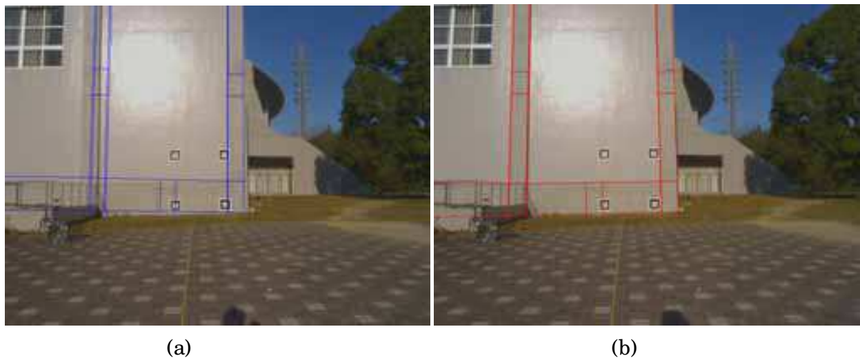
Fig. 17. (a) Captured image of the wall and virtual CG structural blue lines in a single marker usage. Although four markers exist, only one marker was recognized. (b) When the four-marker method was used, the red lines had good agreement.
