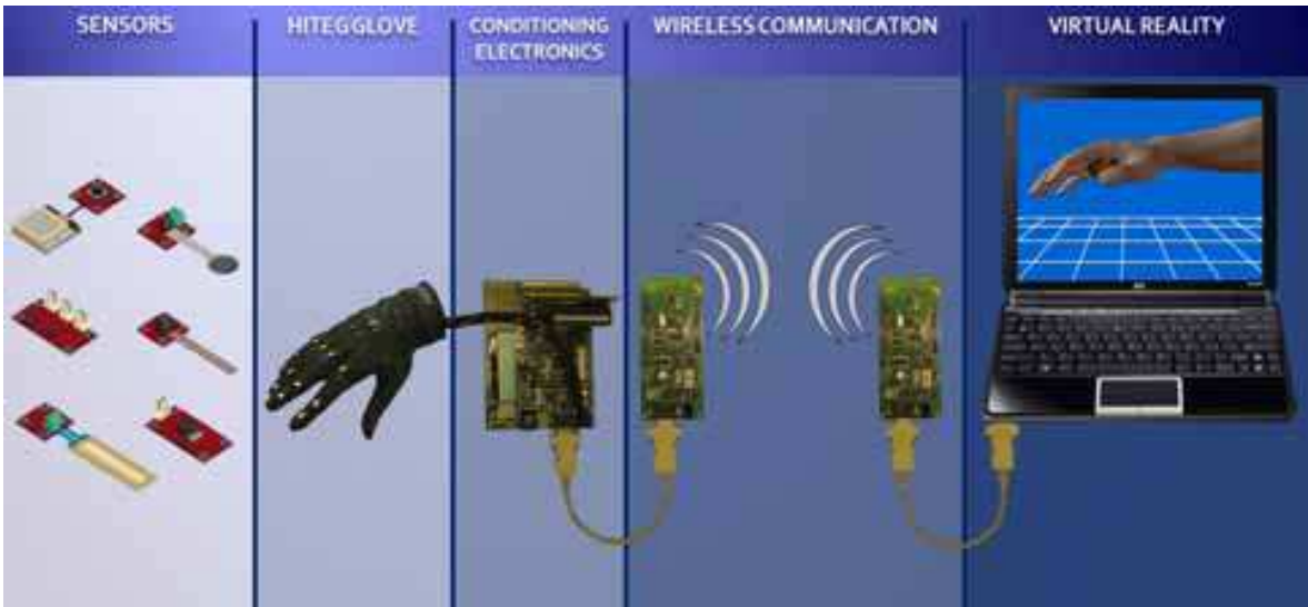
Fig. 20. A schematization of the overall system made of sensors, Hiteg glove, electronic for conditioning the signals, wireless communication board based on ZigBee protocol, and Virtual Reality reproduction
