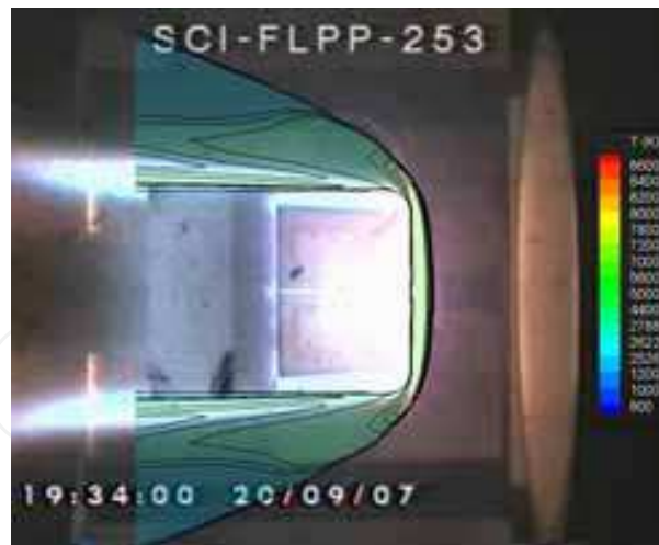
Fig. 35. Top view of the model during test. Comparison with predicted temperature contours
