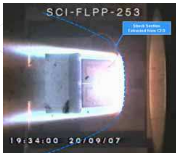
Fig. 34. Top view of the model during test. Comparison of predicted and actual shock shape
