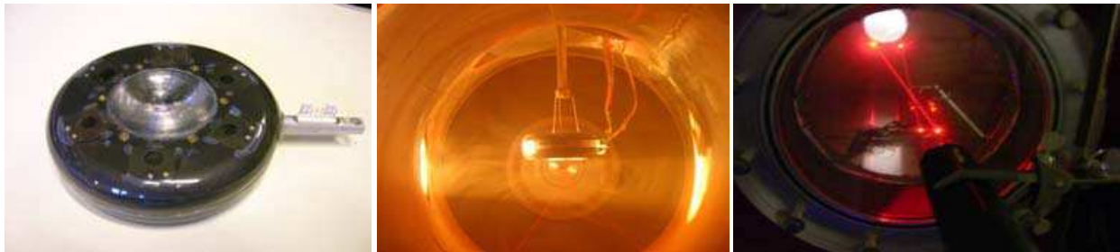
Fig. 8. Photographs of Laser Anemometers (acting also as suspended dust sensors), Left prototype time of flight instrument, Center the sensor during aerosol testing in an environmental wind tunnel, Right A commercial Laser Doppler Anemometer operating through an environmental wind tunnel access window, note the beams illuminating the suspended dust in the flow.
